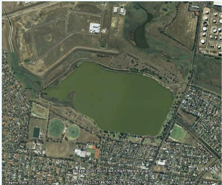
Figure 2. Cherry Lake in Melbourne's southwest was a natural wetland prior to European settlement. Subsequently, it has been partly drained and modified due to pressure from urban development and is now in use as a retarding basin to protect the local community from flooding (Google Earth 2013).
